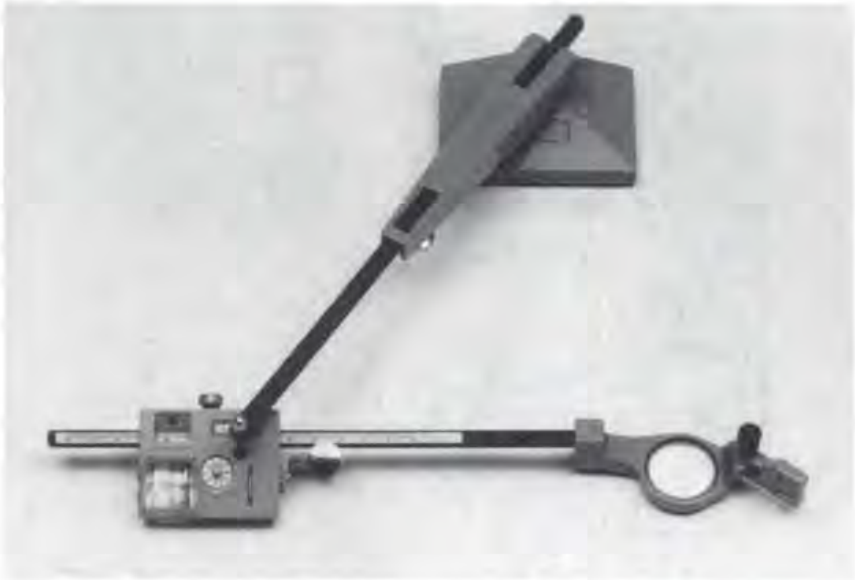
FIGURE 12.6 Mechanical planimeters are normally preferred when occasional use is required.
